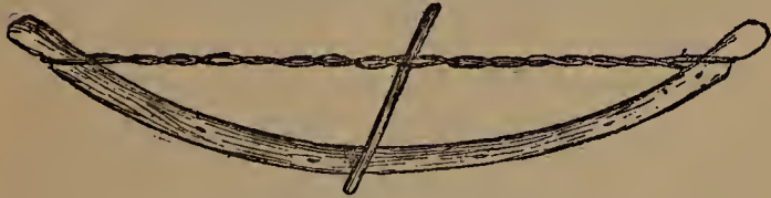
Fig. 54.—Spanish Windlass (for bending wood)
